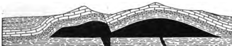
FIG. 11.—Section of Kelly Hill laccolith, Montana. (Same ref. as for Fig. 10, p. 499.) Solid black , porphyry of laccolith; upper broken lines , Mesozoic strata; larger rectangles , Carboniferous; smaller rectangles , Siluro-Devonian; lower broken lines , Cambrian.
